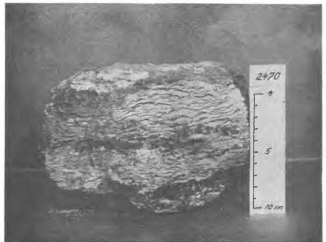
Photograph of clay soil sample No. 2470 from frost heave. Heavy icelenses in centre and below
