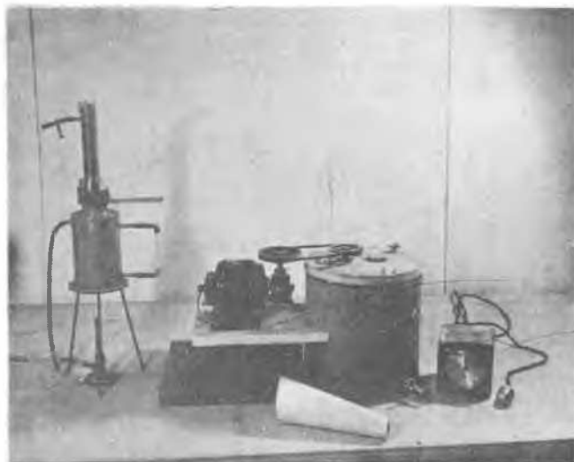
Steam bath and calorimeter for specific heat tests.
