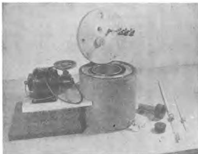
Calorimeter with top off. soil dipper at right.
