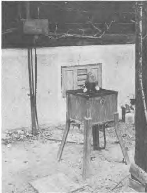
Apparatus for determination of settlement and heaving of surface of soil in dependance of ground-water level.
