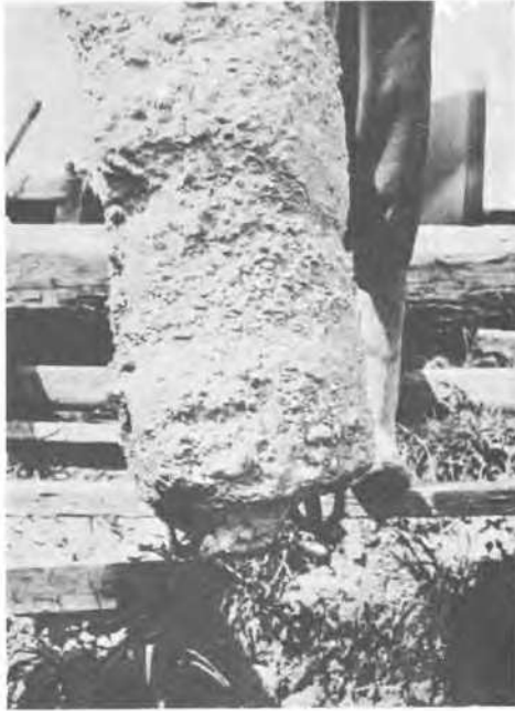
Base of the extracted pile No. 10.
