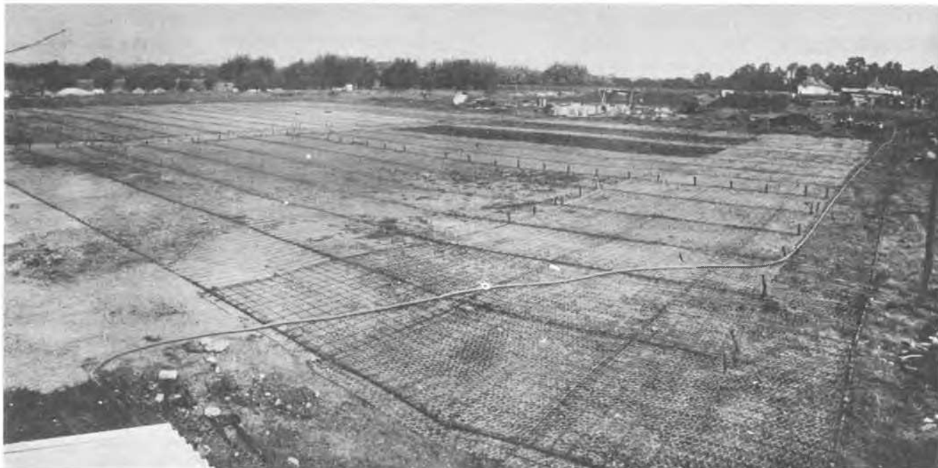
General layout of test site for full-scale steel-distribution tests on square-mesh surfacings
