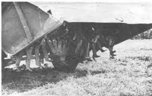
Tines of soil - mixer showing central level gear and depth control shoe.
