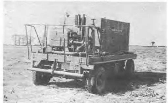
1,000 gallon capacity trailer water sprayer, with 8 H.P. motor pump 6 ft. spraybar piping valves and gauges.
