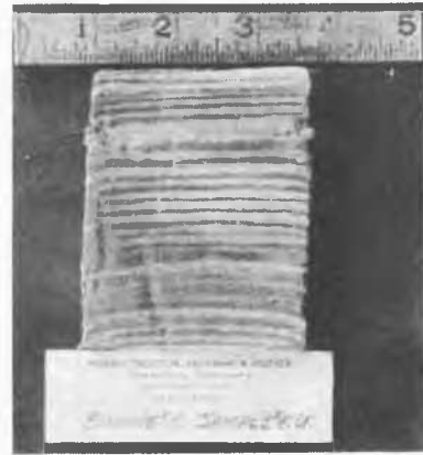
b. Same varved clay recovered with sampler (b) figure 1
