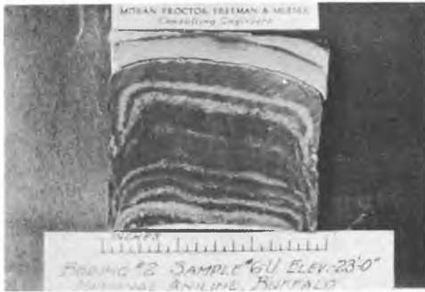
a. Varved clay recovered with sampler (a) figure 1
