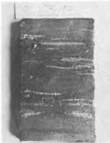
c. Very soft river mud recovered with sampler (c) figure 1
