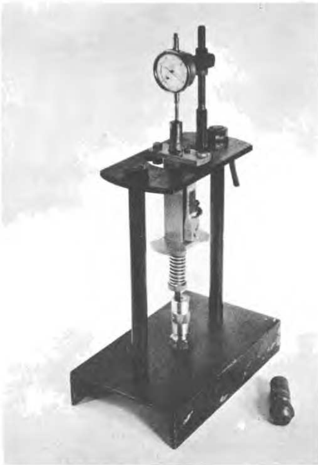
Cantilever deflection gage calibration rack
