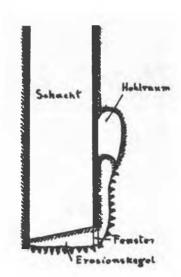
tures through the walling and was located in a height of 15 to 20 m above the upper edge of the window. (See illustration). Such erosions are found also at the foot of clay layers formed as the result of a slide, in which case mostly springs emerge having considerable hydraulic gradients, which may lead to the for-mation of hollows if the deposits of eroded material is continually removed as e.g. by a river.
