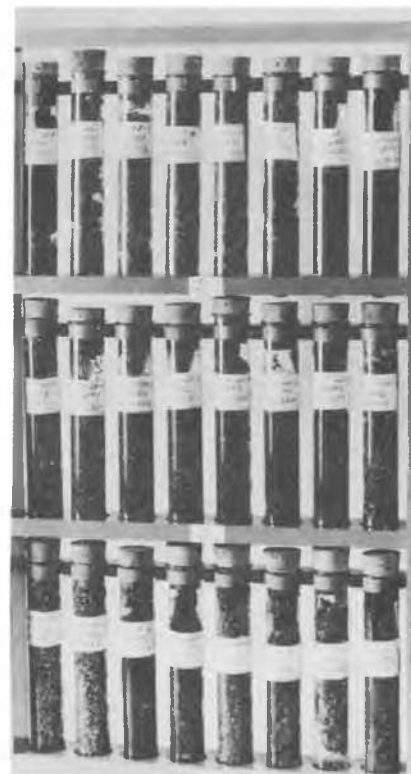
Fig. 6. Illustrating the method used in preserving samples collected at proposed bridge sites. Trays fit in conventional correspondence files.
