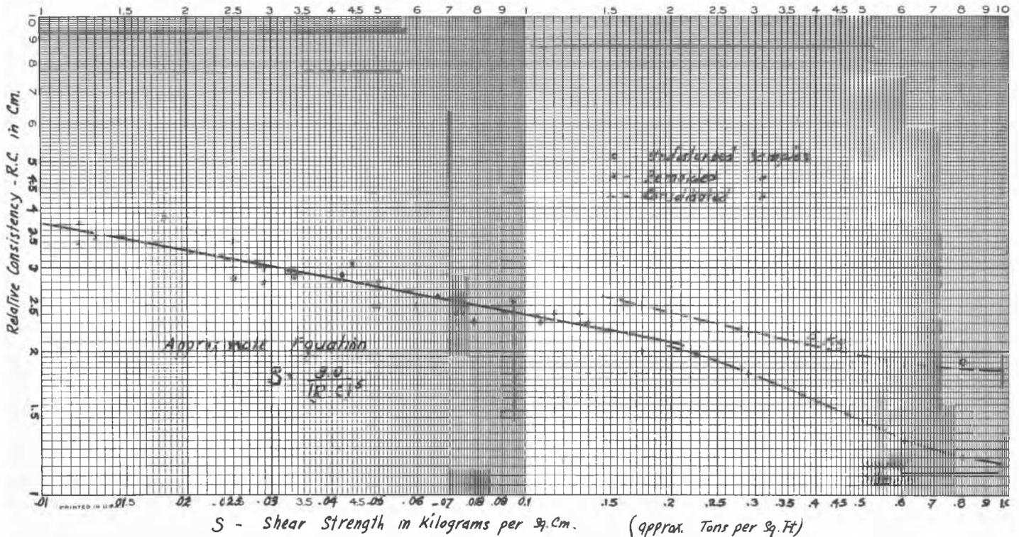
FIG. 8 Approximate Relation between Relative Consistency and Shear Strength of Clays.
