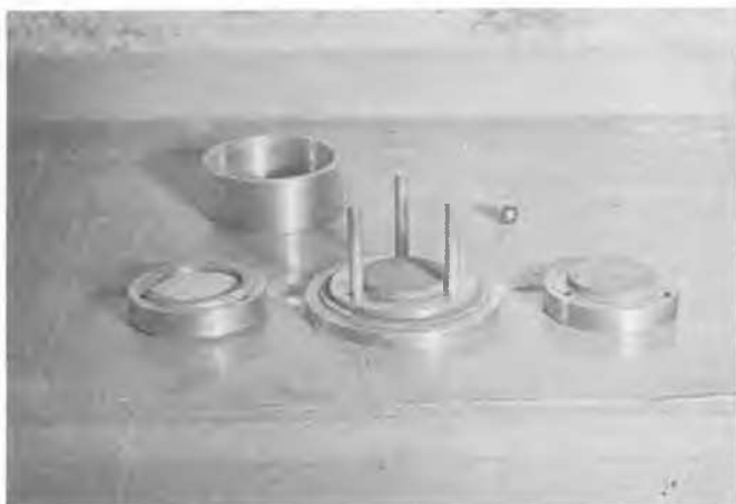
Fig.3. Consolidation Device Dismantled.
