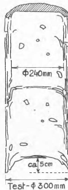
Fig. 7 (above). Defoliation of a core from moraine clay after drying.
