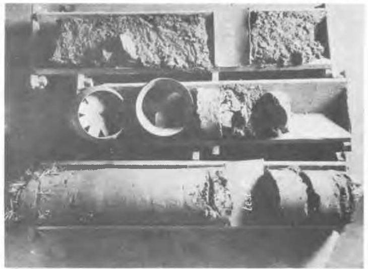
Fig. 9 Whole core (test 25) and dissected core (test 26) Obtained with driving shoe without an inner angle.
