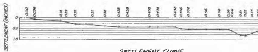
LOADING TEST ON SVAGR PILE
