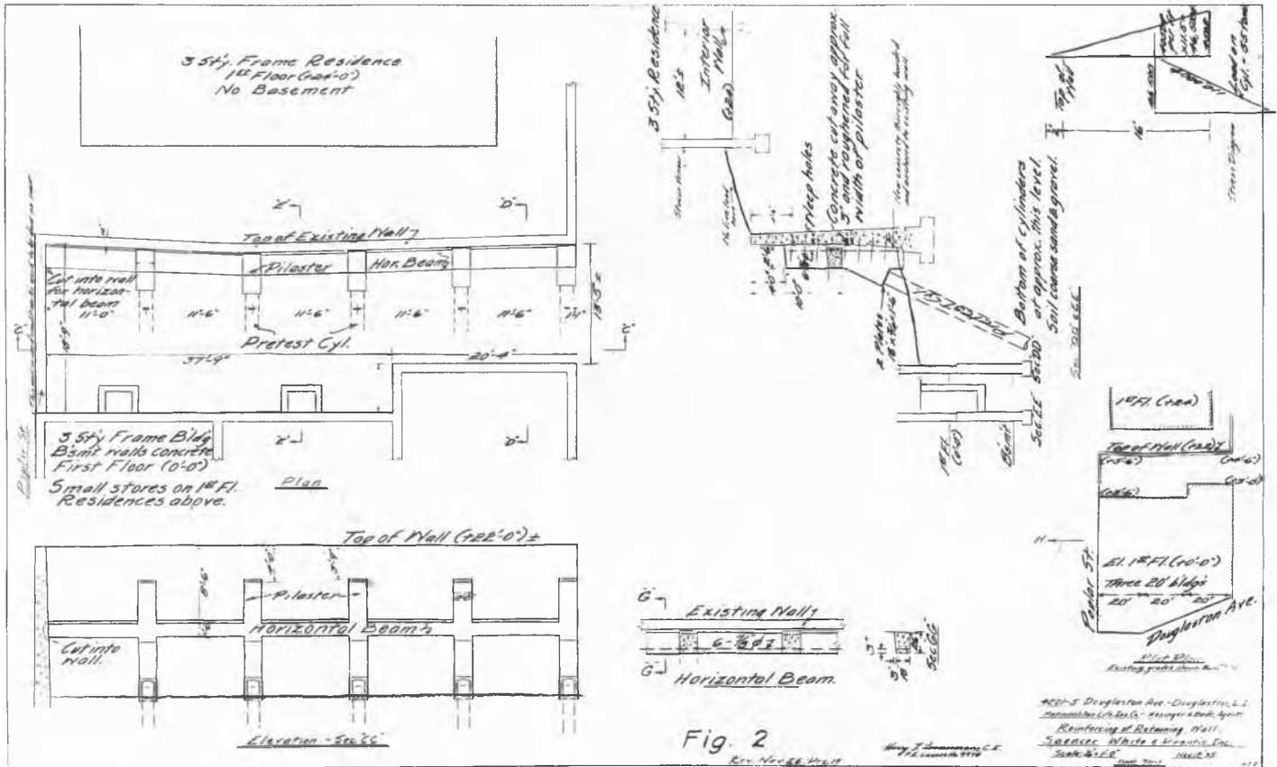
well as to reinforce the wall between the points of application of the cylinder reactions. In order to provide resistance to uplift of the grillage system, the portions of the wall in contact with the vertical supports were roughened, and dowels placed as shown in Fig. 2.
