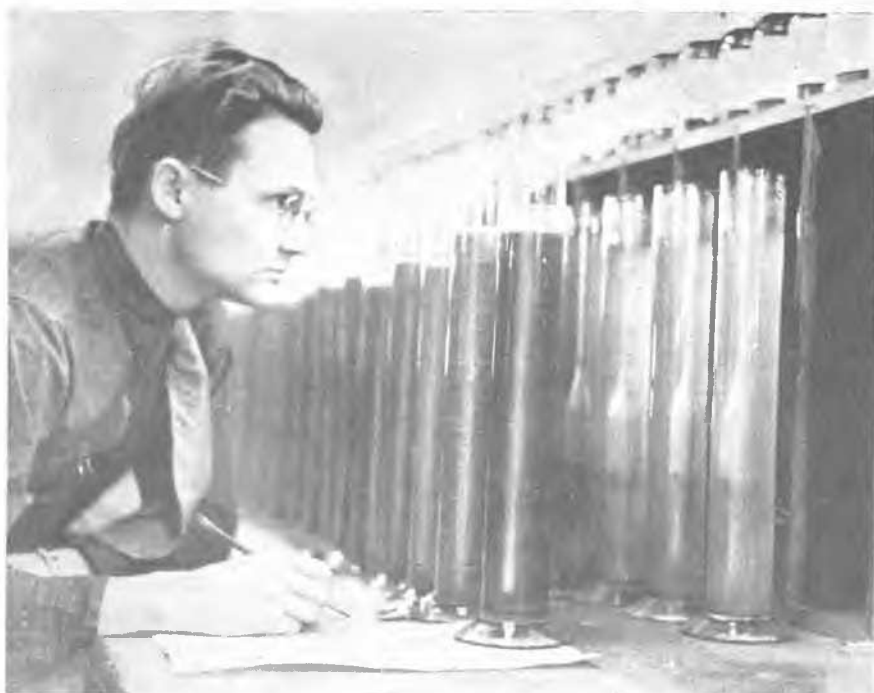
FIG. 1—IN THE SOILS-MECHANICS LABORATORY of the Muskingum flood-control project, different sizes of hydrometers are used to assure accurate determinations at different densities. Soil classification is determined by both sieves and hydrometers.
