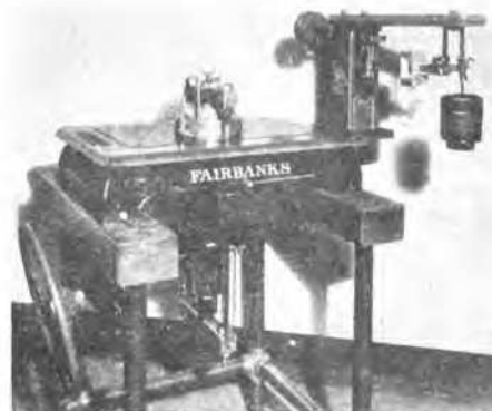
FIG. 2—A JACK combined with a modified platform scale proves a convenient loading rig for both consolidation and shear tests.
