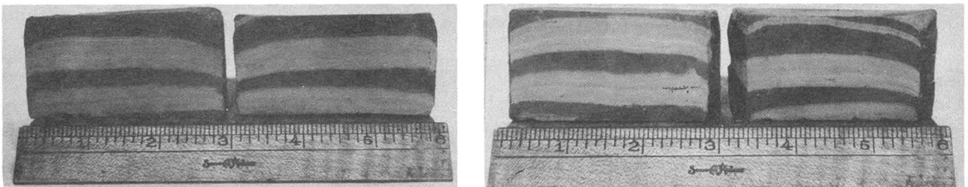
Fig. 1 Distortion of Sample as a Result of Frictional Drag within the Sampling Tube
