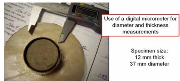
Figure 11: Measurement of the “Shrinkage Curve”, SC using micrometer calipers
