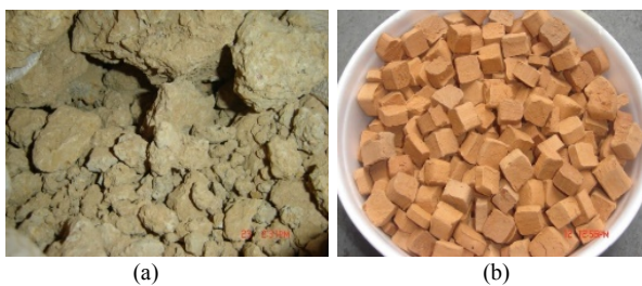
Figure 5. Production process of SCACC: (a) natural clayey soil, and (b) after burnt at 850 °C (Campos et al. 2017)
