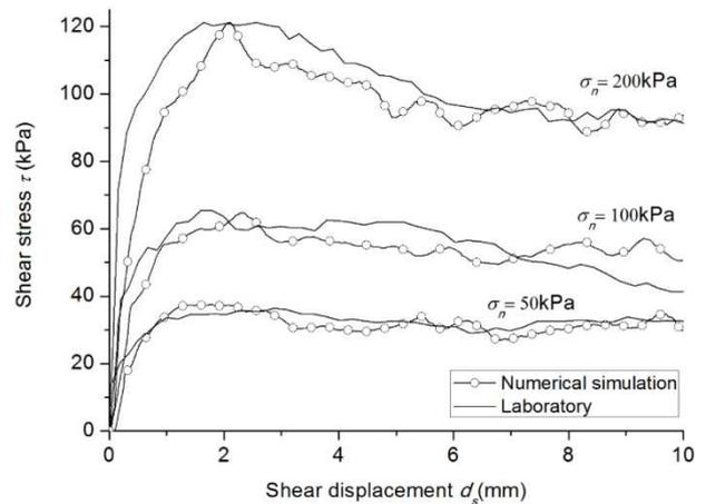
Figure 5. Shear stress versus shear displacement in laboratory testings and in numerical simulations
