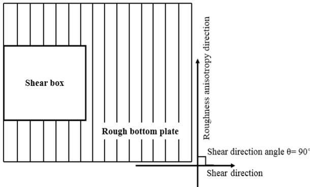
Figure 2. Overhead view of the numerical interface shear test ( $\theta = 90^\circ$ )
