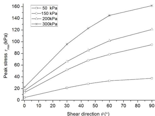
Figure 8. Peak stress against angles of shear direction for various normal degree of stress
