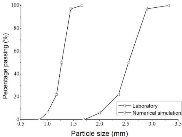
Figure 4. Particle size distributions in laboratory testing and in numerical simulation
