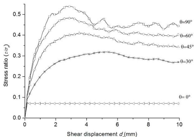
Figure 6. Stress ratio ( $\tau/\sigma_n$ ) with respect to shear displacement for various angles of shear direction ( $\sigma_n = 300$  kPa)
