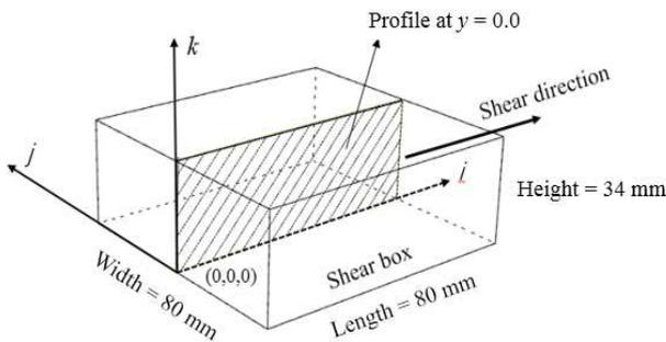
Figure 3. Schematic diagram of the shear box in the local coordinate of the shear box
