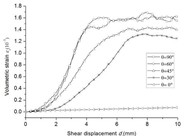
Figure 7. Volumetric strain with respect to shear displacement for various angles of shear direction ( $\sigma_n = 300$  kPa)
