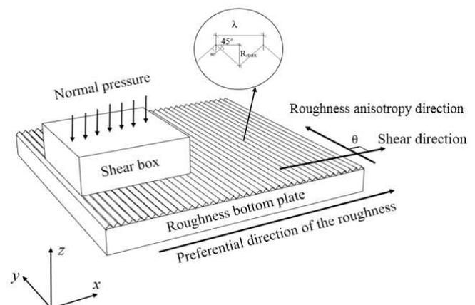
Figure 1. Schematic diagram of the numerical interface shear test
