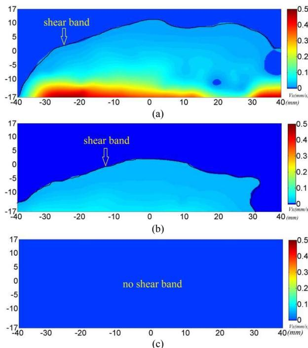
Figure 9.  $x$ -direction velocity distribution field of particles at  $d_s = 2.5$ mm ( $\sigma_n = 300$  kPa): (a) at  $\theta = 90^\circ$ ; (a) at  $\theta = 45^\circ$ ; (c) at  $\theta = 0^\circ$
