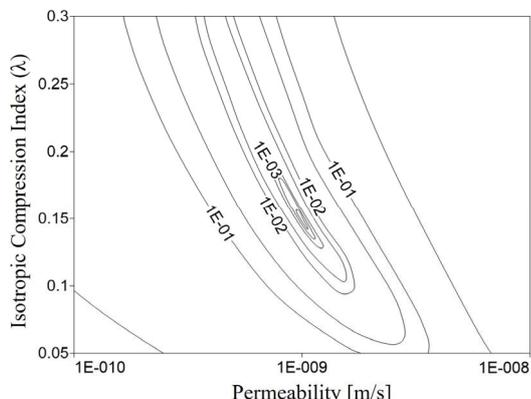
Figure 2. Objective function ( $J$ ) defined only using vertical displacements ( $U_y$ ) 1 month after applying the preloading.
