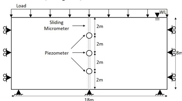
Figure 1. Synthetic case study geometry. WL: Water Level.
