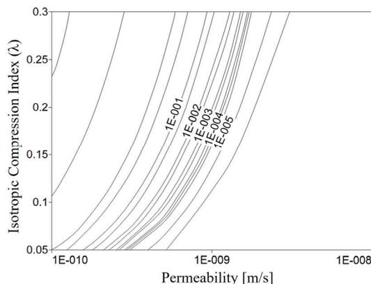
Figure 5. Objective function ( $J$ ) defined only using pore water pressure ( $P_w$ ) 10 years after applying the preloading.
