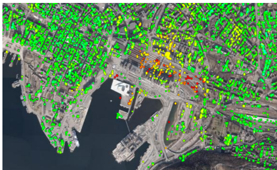
Figure 1. A processed satellite image giving average annual displacement rates (velocity) in central part of Oslo, Norway ( https://maps.globesar.com/ ).
