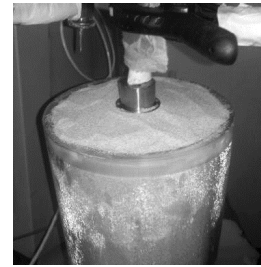
Figure 2. Receiver bender element inserted in the specimen.
