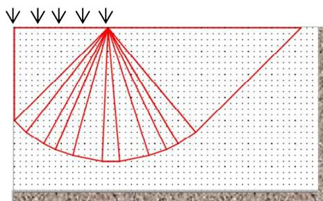
Figure 7. Required nodal density to achieve a similar accuracy to the result in Figure 6 using a uniform starting nodal grid with standard member adding (solution  $N_c = 5.15$ , 1537 nodes)
