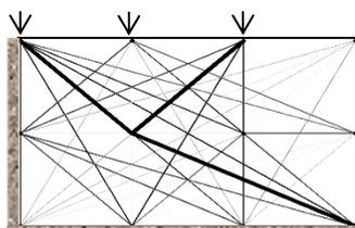
Figure 2. Dual equilibrium output for example problem in Figure 1 (slip-line grey-scale and width both used to represent shear stress magnitude. Black indicates yielding, white indicates zero shear stress).
