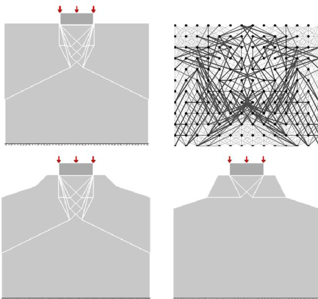
Figure 8. (a) Problem of foundation on vertically sided ‘embankment’ using Limit State GEO (b) low stressed squares identified in DLO solution. (c) modified geometry based on (a) removing low stressed areas. (d) Different failure mechanism due to removing material from higher stressed zones.
