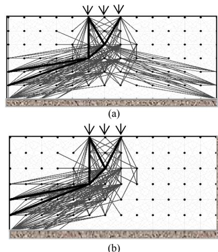
Figure 4. Dual equilibrium output for example problem (a) potential sliplines >80% yield in grey and critical mechanism in black (b) Same problem as (a) with right side constrained.
