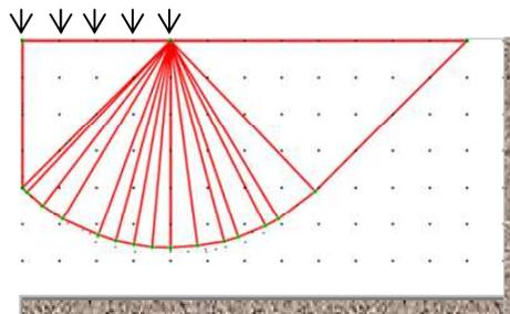
Figure 6. Solution of Prandtl punch problem in a unit cohesion soil (symmetric half space) using adaptive nodal addition (solution  $N_c = 5.15$ , 167 nodes)
