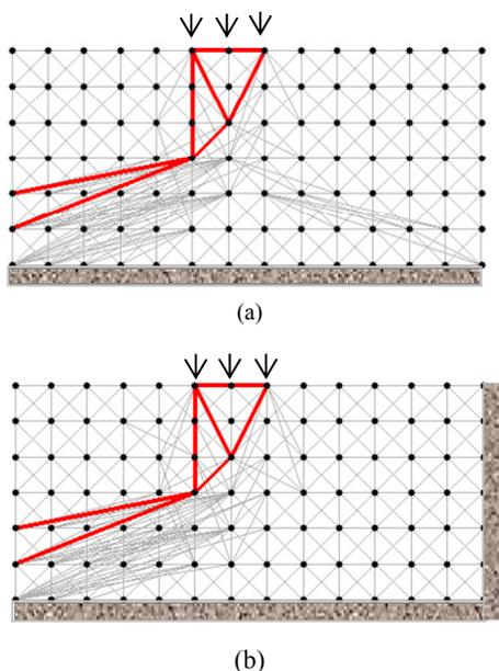
Figure 5. Member adding lines for example problem (a) member adding lines in grey and critical mechanism in black (b) Same problem as (a) with right side constrained
