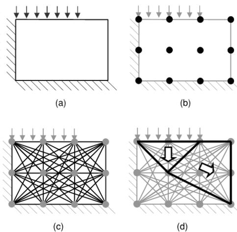
Figure 1. Stages in DLO procedure (after Gilbert et al. (2010)): (a) initial problem definition (surcharge applied to block of soil close to a vertical cut); (b) discretization of soil using nodes; (c) interconnection of nodes with potential discontinuities; (d) identification of critical subset of potential discontinuities using optimization (giving the layout of slip-lines in the critical failure mechanism).
