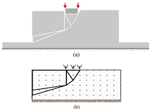
Figure 3. Example problem of foundation on vertically sided ‘embankment’, (a) failure geometry and mechanism generated using Limit State: GEO. (b) schematic nodal layout.
