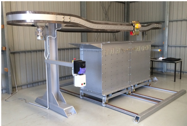
Figure 2. Test rig for scale model impact roller.
