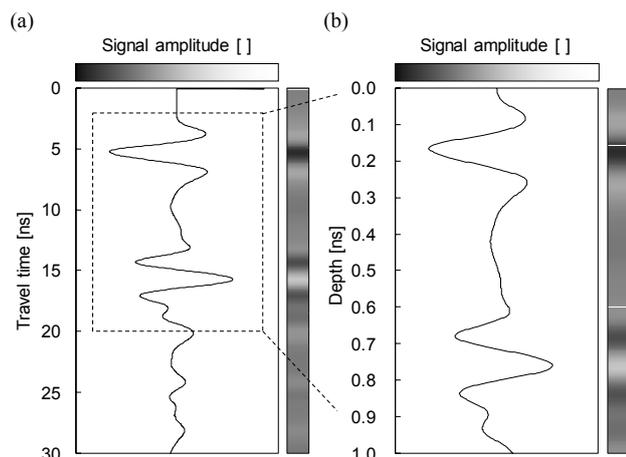
Figure 5. GPR signals: (a) GPR signal in temporal scale; (b) GPR signal in spatial scale.
