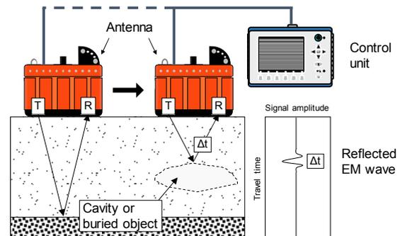
Figure 1. Measurement system of the ground penetrating radar. T and R are the transmitter and receiver, respectively; EM denotes the electromagnetic wave;  $\Delta t$  is the travel time of the electromagnetic wave reflected at an interface in the ground.
