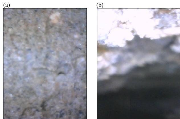
Figure 3. Endoscopic images: (a) Endoscopic image taken at the ground specimen; (b) Endoscopic image taken at the interface between the ground specimen and the cavity.
