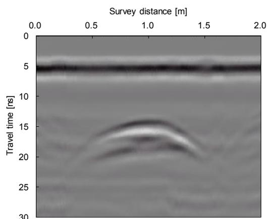
Figure 4. GPR image in temporal scale.
