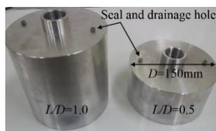
Fig. 2. Photos of bucket foundations used in this study
