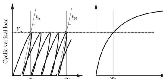
Fig. 5. Definition of accumulated vertical pullout displacement and unloading stiffness
