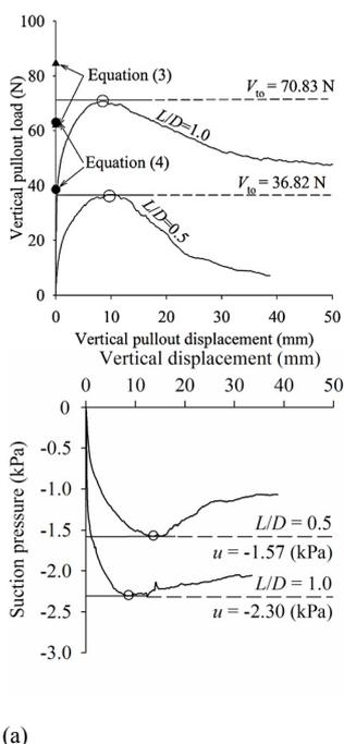
Fig. 3. Static vertical pullout test results: (a) load-displacement curves and (b) development of suction pressure
