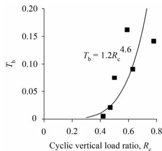
Fig. 6. Variation of  $T_b$  parameters at different  $R_c$  values for saturated sand
