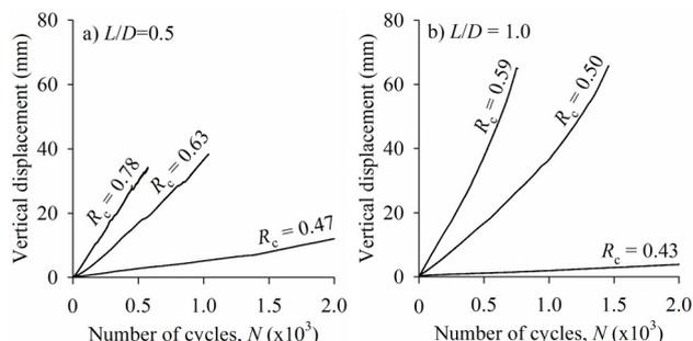
Fig. 4. Accumulated pullout displacement at different cyclic load magnitudes
