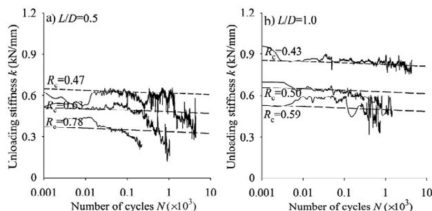
Fig. 7. Unloading stiffness at different load magnitudes
