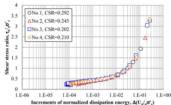
Figure 19. Relationship of shear stress ratio and normalized dissipation energy in a logarithm scale.
