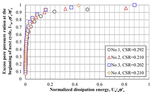
Figure 17. Relationships of normalized dissipation energy and excess pore pressure ratio at the beginning of next cycle.
