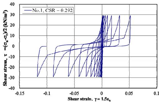
Figure 2. Stress-strain relationship in No.1.
