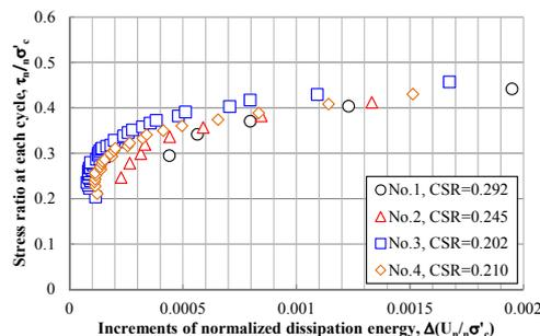
Figure 15. Magnified view of the relationship of shear stress ratio and normalized dissipation energy in early stage of tests.
