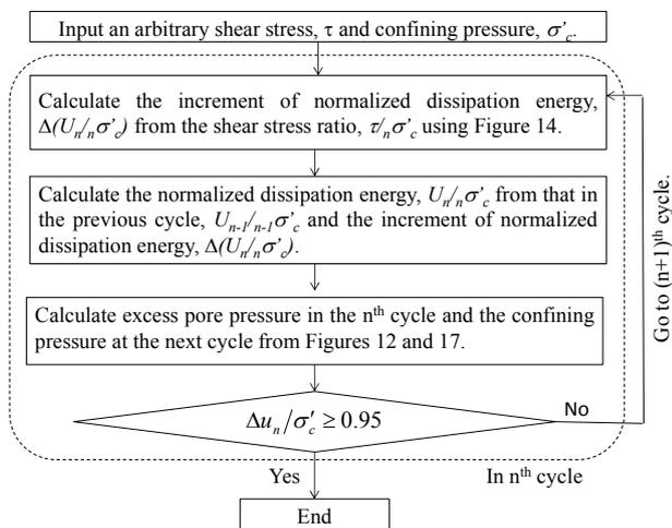
Figure 16. Flow chart to calculate a liquefaction strength curve using a cyclic undrained triaxial test.
