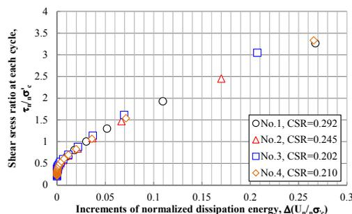
Figure 14. Shear stress ratios and increments of normalized dissipation energy using confining pressure at the beginning of each cycle.
