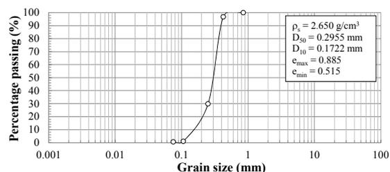
Figure 1. Grain size distribution curve of Iide silica sand (No.6).
