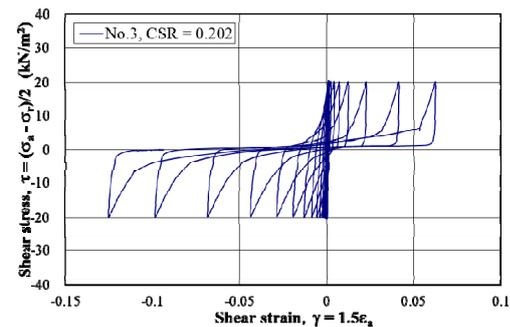
Figure 4. Stress-strain relationship in No.3.
