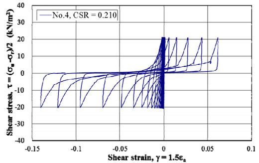
Figure 5. Stress-strain relationship in No.4.
