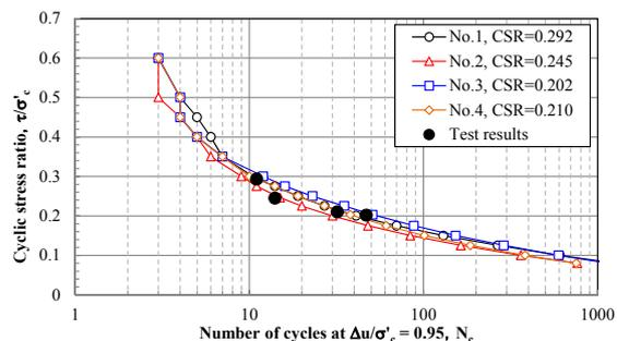
Figure 18. Estimated liquefaction strength curves and test results of cyclic undrained triaxial tests.
