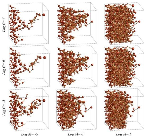
Figure 3. Selected simulations for different pairs of Log M and Log C numbers for tube size distribution case II (standard deviation =  $1\sigma$ ). The fluid flow direction is from the left to the right boundary.
