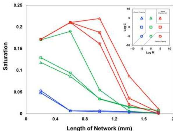
Figure 4. Saturation of invading fluid for different LogM and LogC numbers in different sections of the pore network model.
