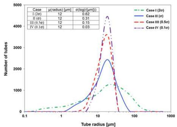
Figure 2. Different tube size distribution used in this study.
