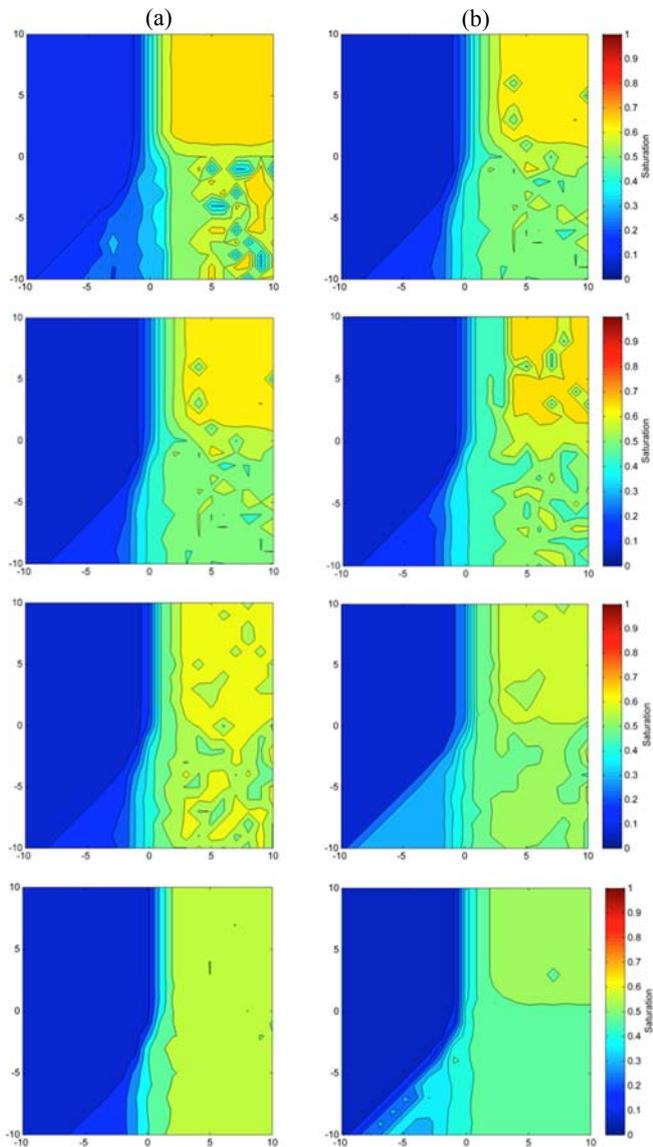
Figure 5. Saturation of invading fluid in Log M-Log C map. (a) Effect of different tube size distributions ( $2\sigma$ ,  $\sigma$  and  $0.5\sigma$  cases, from top to bottom). (b) Effect of connectivity for different coordination numbers  $cn=8.0$ ,  $cn=6.2$ ,  $cn=5.1$  and  $cn=4.6$  (from top to bottom).
