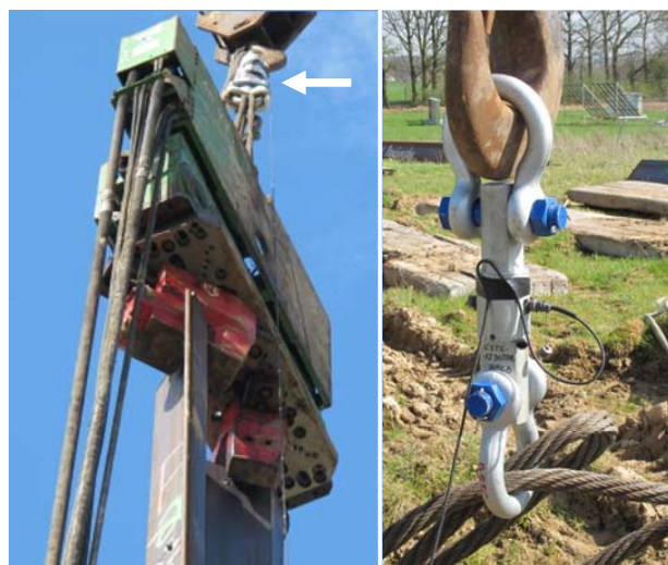
Figure 4. BBRI holding back force transducer as used during the test campaign
