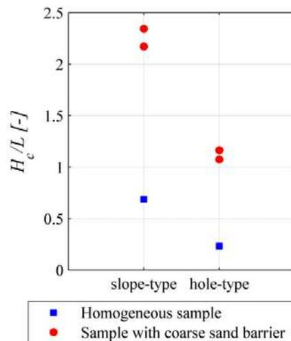
Figure 2. Critical gradients obtained in the experiments
