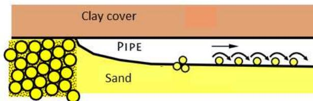
Figure 1. Principle of the coarse sand barrier
