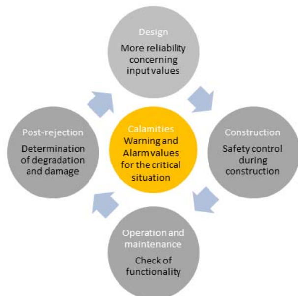
Figure 1. Life cycle of a dike indicating the role of monitoring in each phase
