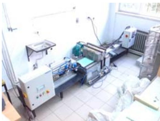
Figure 4. Large displacement large size direct shear testing device (Baykal 2016).
