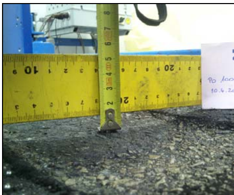
Figure 7. View of the rut which developed under the loading wheel at the end of the test.
