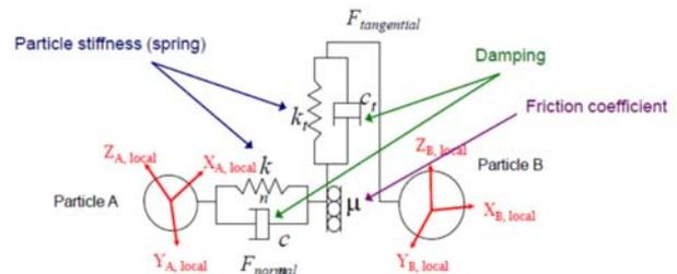
Figure 1. Schematic diagram for Hertz-Mindlin contact model [6]
