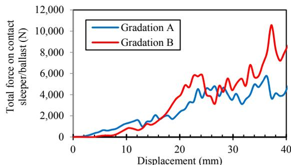
Figure 6. Total contact force acting at sleeper/ballast interface
