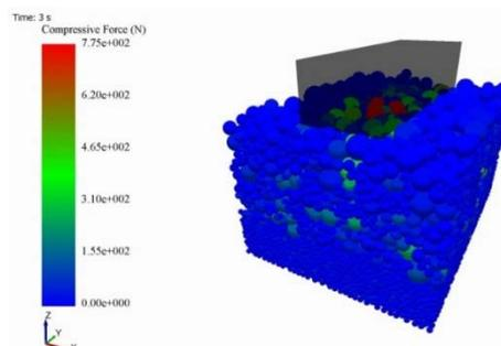
Figure 7. Compressive force of particles at time period of 3 seconds
