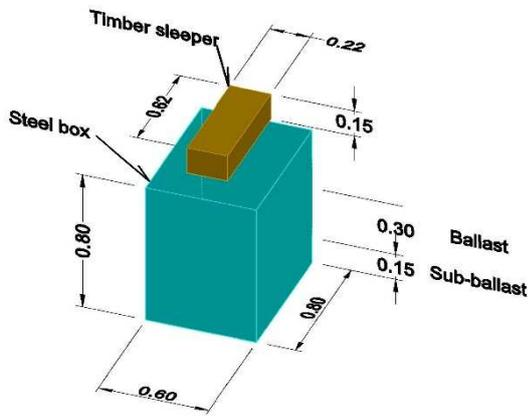
Figure 2. Schematic illustration of triaxial chamber
