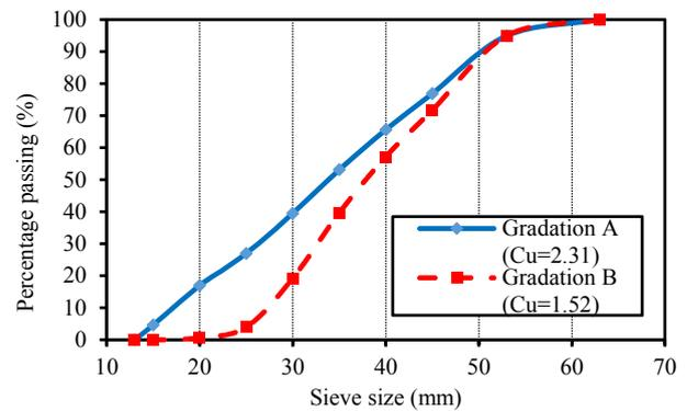
Figure 3. Particle size distribution curve for ballast material
