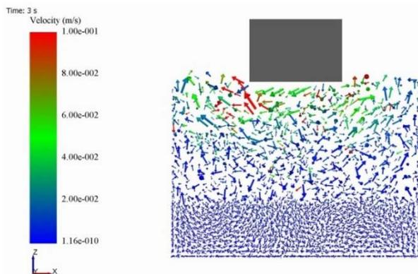
Figure 9. Velocity vectors of railway ballast during loading
