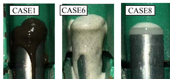
Figure 8. Typical boiling sand results.
