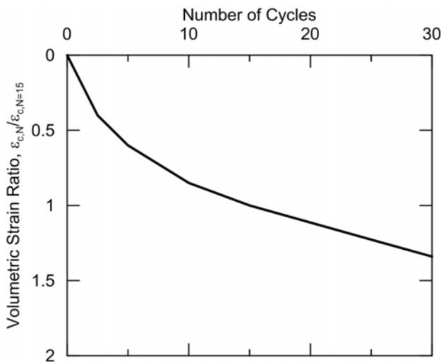
Figure 2. Relationship between volumetric strain ratio and number of cycles for the simplified procedure (reproduced from Tokimatsu and Seed 1987).
