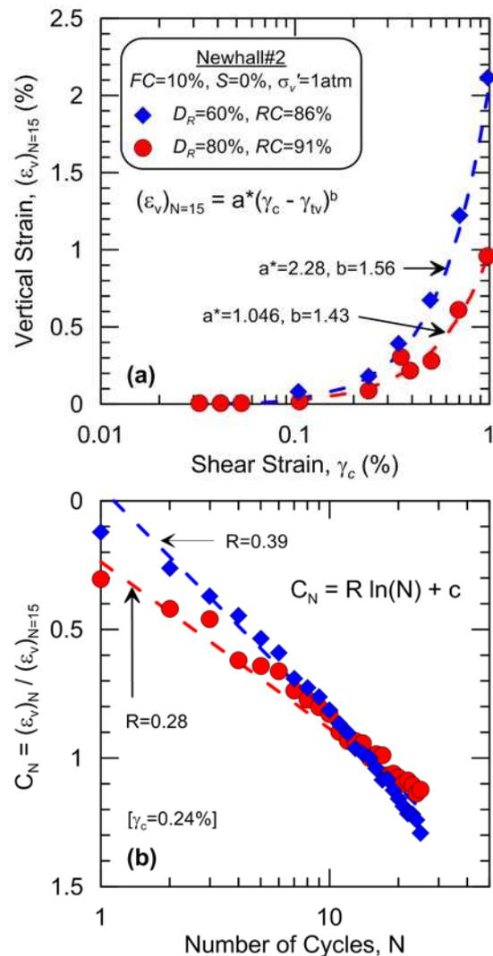
Figure 3. Components from a VSMM (taken and modified from Yee et al. 2014). (a) Vertical strain vs. shear strain and (b) normalized vertical strain vs. number of cycles.
