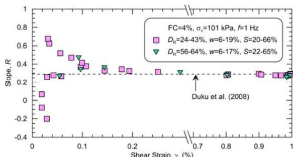
Figure 5. Variation of parameter  $R$  against shear strain in a VSMM considering changes in relative density.
