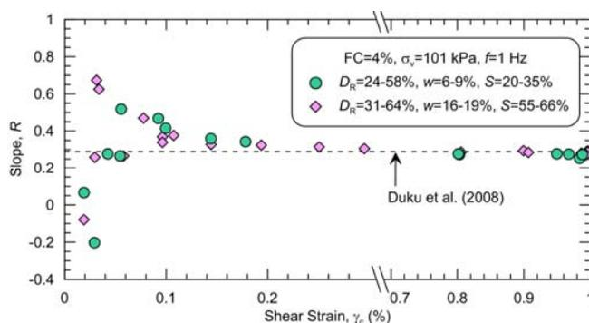
Figure 6. Variation of parameter  $R$  against shear strain in a VSMM considering changes in saturation.
