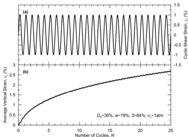
Figure 4. Sample digitally controlled simple shear testing of a sandy material. (a) Cyclic shear strain cycles and (b) average vertical strain vs. number of cycles.
