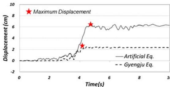
Figure 4. Pile displacement.
