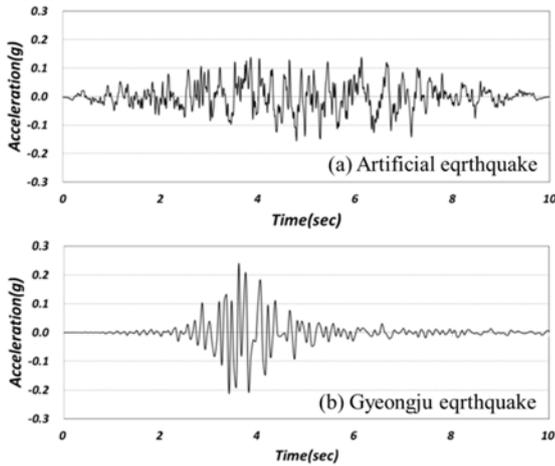
Figure 2. Artificial and Gyeongju earthquakes.
