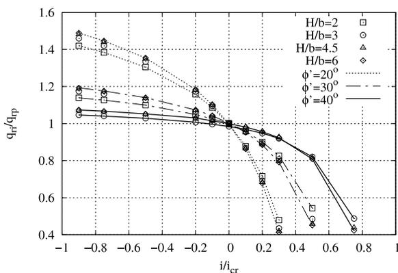
Figure 6: Ratio between the bearing capacity obtained for the impervious and pervious footing for all cases.
