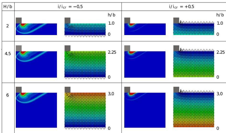
Figure 4: Impervious footing: plastic strains, hydraulic heads and seepage forces for  $\phi'=30^\circ$ ,  $H/b=2, 4.5$  and  $6$ , and  $i/i_{cr}=\pm 0.5$ .
