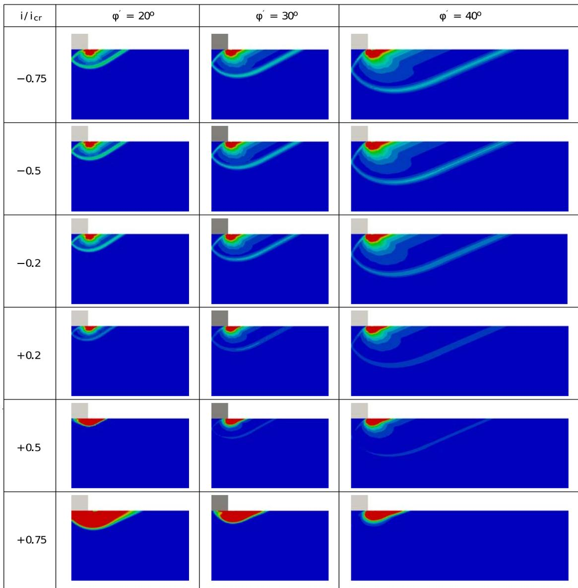
Figure 5: Impervious footing: plastic strains, hydraulic heads and seepage forces for different values of  $\phi'$  and  $i/i_{cr}$ , for  $H/b=4.5$ .
