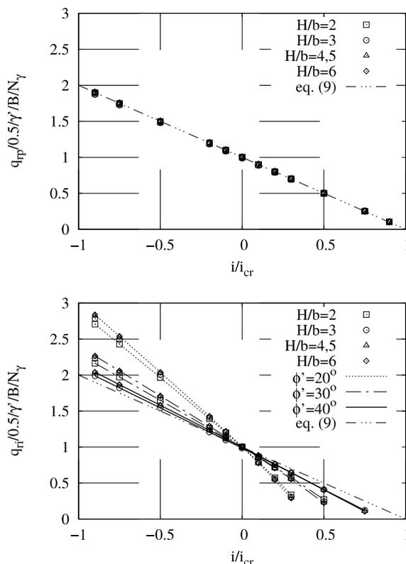
Figure 2: Dimensionless bearing capacities determined from the calculations, using the values of  $N_g$  obtained for pervious footing
