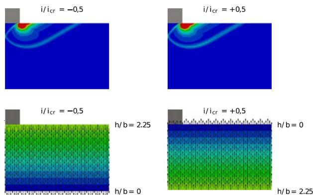
Figure 3: Pervious footing: plastic strains, hydraulic heads and seepage forces for  $\phi' = 30^\circ$ ,  $H/b = 4.5$  and  $i/i_{cr} = \pm 0.5$ .
