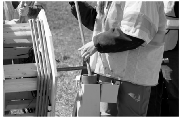
Figure 5. Installation of SAAV into an existing inclinometer casing.
