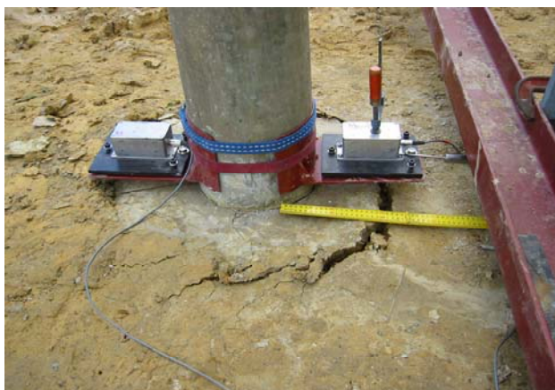
Figure 1. Ground surface around a pole shaft near the end of the lateral loading. Note the embedment concrete and the gap which has opened behind.
