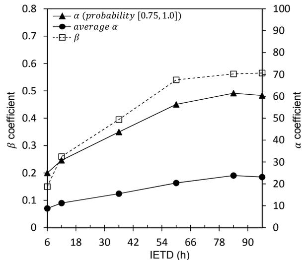
Figure 3. Changes in coefficients  $\alpha$  and  $\beta$  with various IETDs
