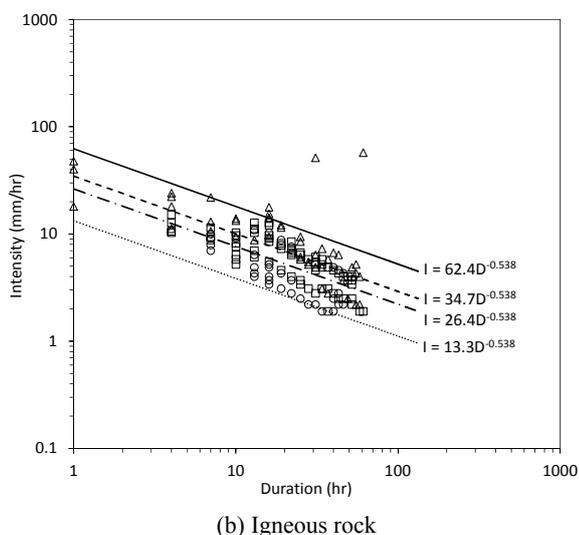
Figure 5. Comparison between two metropolitan ID curves for metamorphic rock and igneous rock
