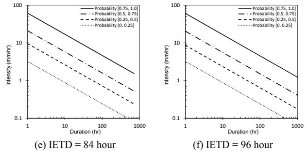
Figure 2. Proposed probabilistic ID curves with various IETDs
