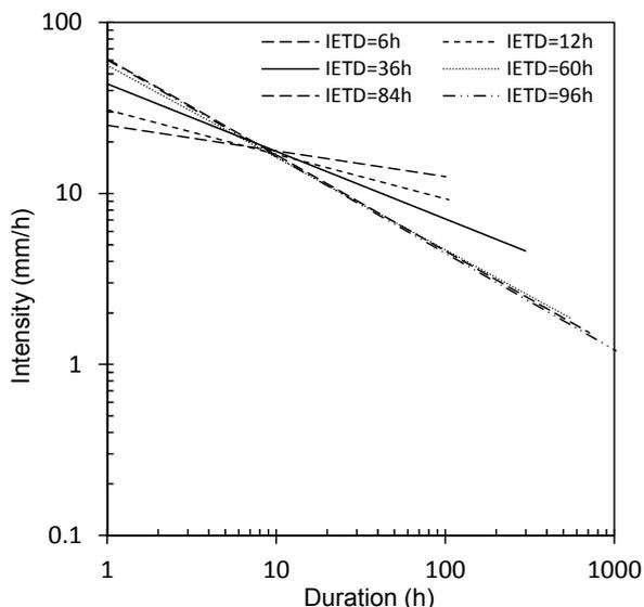
Figure 4. ID curves corresponding to the probability of landslide occurrence 0.75 ~ 1.0
