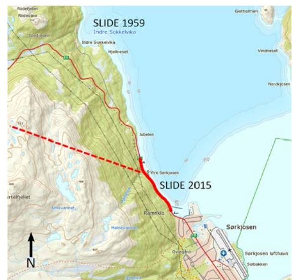
Figure 1. Soerkjosen is 75 km east of the city of Tromsø in Norway. The 2015 slide sent the shoreline marked by a solid line into the fjord. The dotted line is a rock tunnel under construction. The site of a disastrous landslide in 1959 in Sokkelvik that killed 9 persons is marked.
