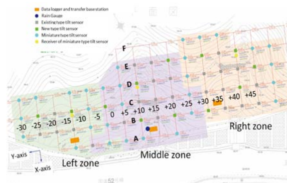
Figure 11. Arrangement of the multi-point tilt sensors
