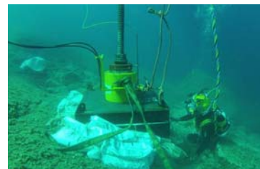
Figure 6. A picture of the test set-up, clearly showing the hydraulic jack
