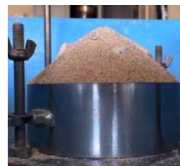
Photo 2. Angle of repose test for coral gravel soil of 10% of gravel content.
