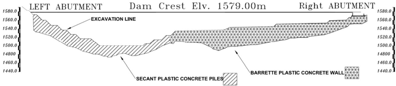
Figure 1. Longitudinal cross section of Silveh dam
