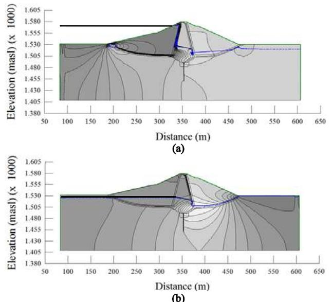
Figure 5. Phreatic and equipotential lines obtained from unsaturated transient seepage analyses; (a) before, and (b) after the first impounding.
