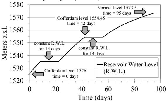
Figure 3. Variation of reservoir water level with time for the proposed first impounding time plan for Silveh Dam
