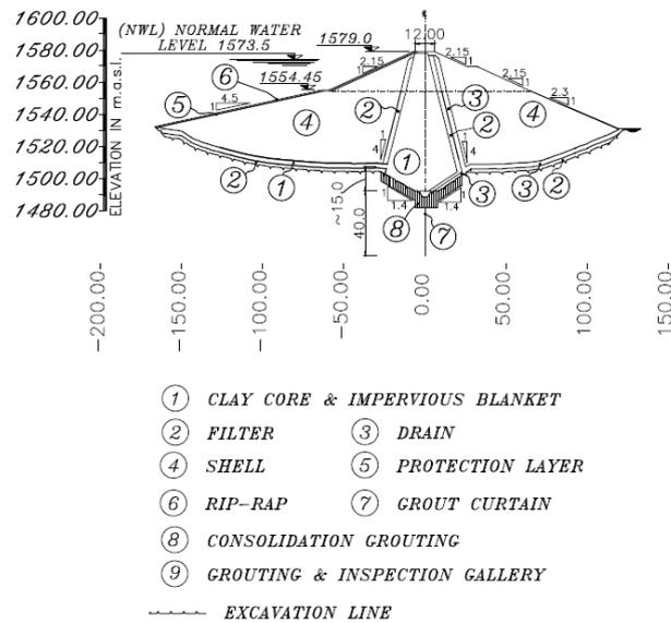
Figure 2. Maximum height cross section of Silveh Dam
