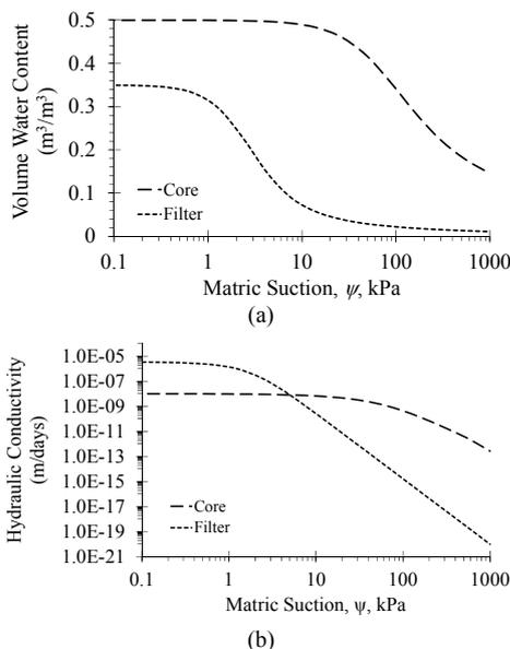
Figure 4. Unsaturated soil parameters of core and filter materials; (a) soil water retention characteristics (SWRC), and (b) hydraulic conductivity curves.
