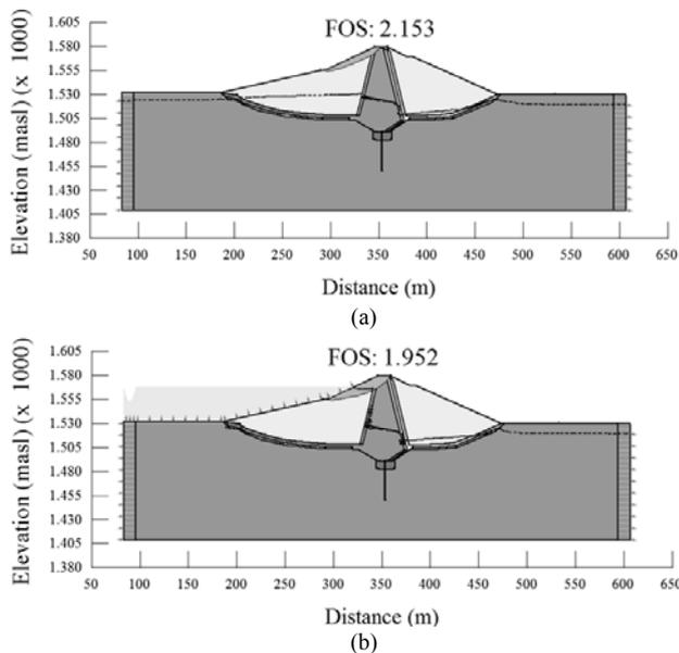
Figure 6. Minimum safety factors obtained from limit equilibrium slope stability analyses; (a) before impounding, and (b) at the critical water level.
