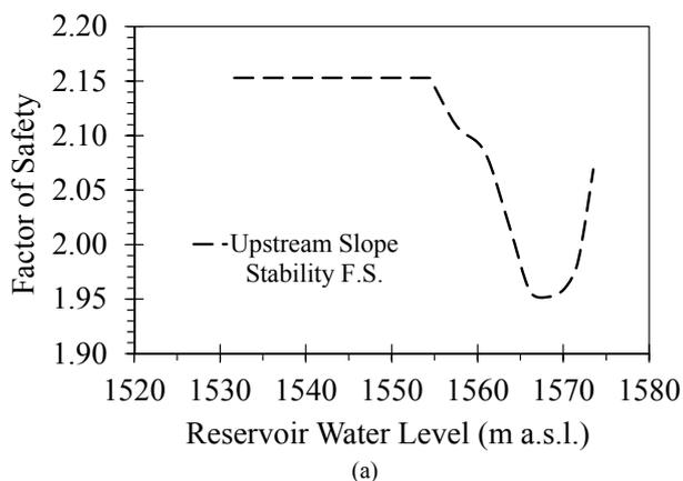
Figure 7. Variation of safety factor against upstream slope instability with reservoir water level.
