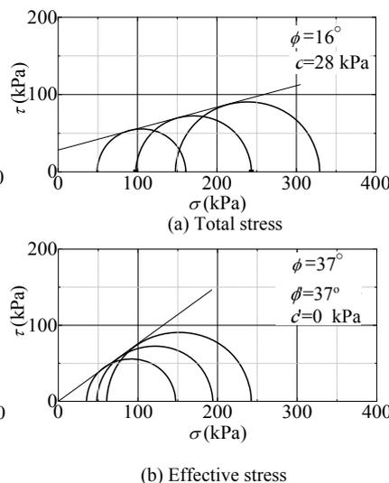
Figure 9. Mohr's stress circle (Method-B)
