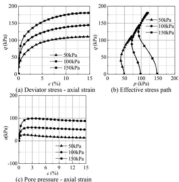
Figure 6: Triaxial test results of the soils collected by Method-B
