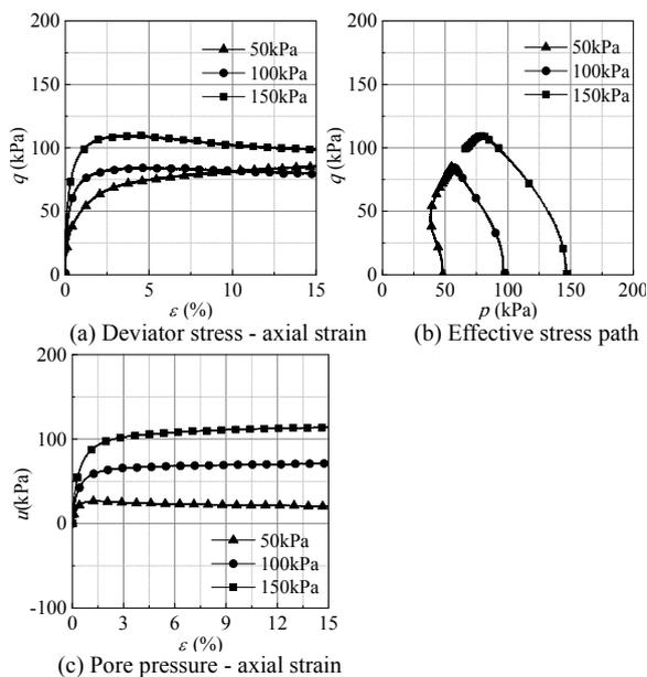
Figure 7: Triaxial test results of the soils collected by Method-B-i
