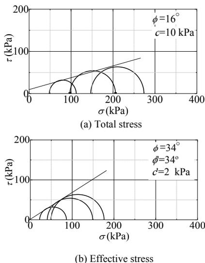
Figure 8. Mohr's stress circle (Method-A)
