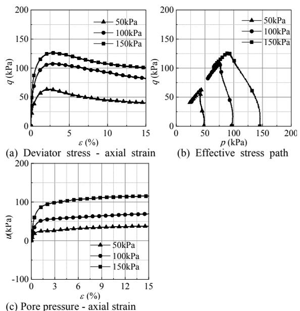
Figure 5: Triaxial test results of the soils collected by Method-A
