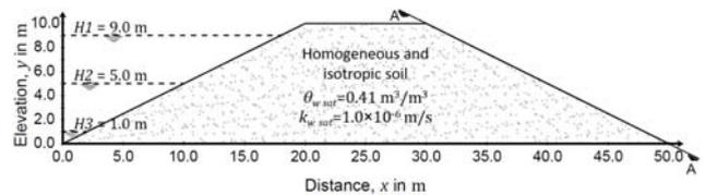
Figure 7. Cross-section of the homogeneous embankment evaluated.
