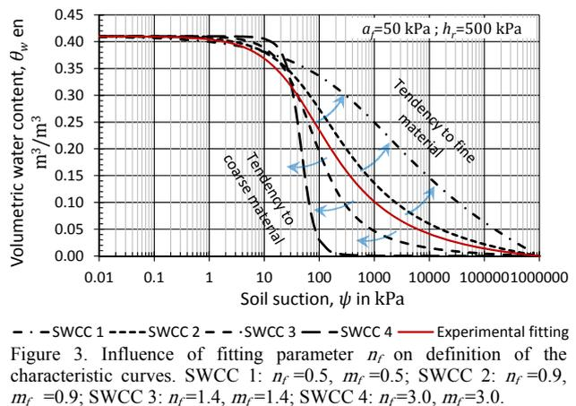
Figure 3. Influence of fitting parameter  $n_f$  on definition of the characteristic curves. SWCC 1:  $n_f=0.5$ ,  $m_f=0.5$ ; SWCC 2:  $n_f=0.9$ ,  $m_f=0.9$ ; SWCC 3:  $n_f=1.4$ ,  $m_f=1.4$ ; SWCC 4:  $n_f=3.0$ ,  $m_f=3.0$ .
