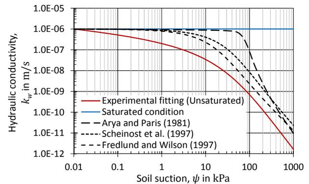
Figure 6. Hydraulic conductivity functions assumed for the analyses.
