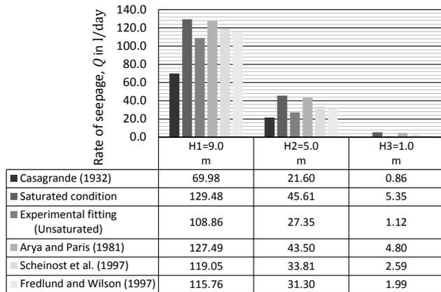
Figure 9. Variation of rates of seepage through the homogeneous embankment for the three water levels evaluated.
