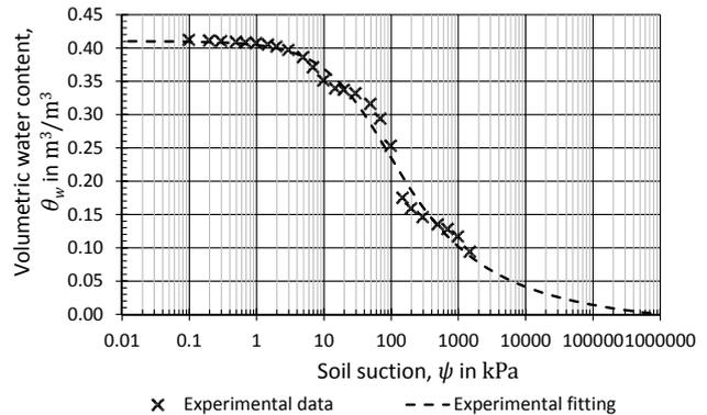
Figure 1. Experimental data and SWCC adjusted by the model of Fredlund and Xing (1994), assumed in calculations.
