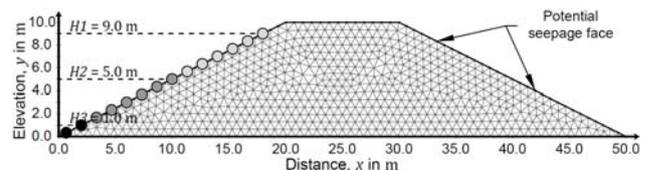
Figure 8. Finite element mesh and boundary conditions assumed in calculations for the homogeneous embankment.
