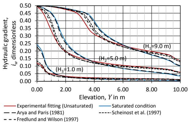
Figure 10. Exit hydraulic gradients (resulting magnitude) in section A-A from the Fig. 7, for the three water levels evaluated.
