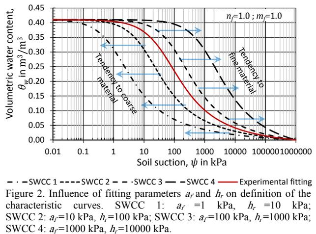
Figure 2. Influence of fitting parameters  $a_f$  and  $h_r$  on definition of the characteristic curves. SWCC 1:  $a_f=1$  kPa,  $h_r=10$  kPa; SWCC 2:  $a_f=10$  kPa,  $h_r=100$  kPa; SWCC 3:  $a_f=100$  kPa,  $h_r=1000$  kPa; SWCC 4:  $a_f=1000$  kPa,  $h_r=10000$  kPa.
